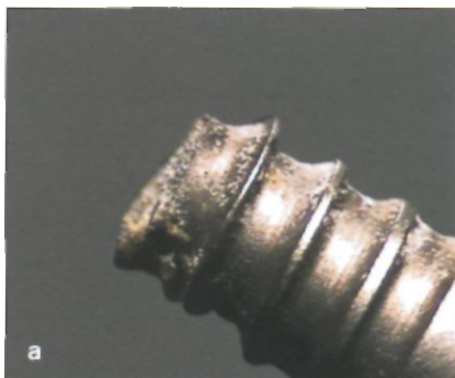
Figs 3-37a and 3-37b Area B in Fig 3-35 can be broken if the insertion angle is changed during implantation at an area where there is hard bone, such as the posterior mandible. It can also be broken by the leverage effect with a contra-angled long driver.
